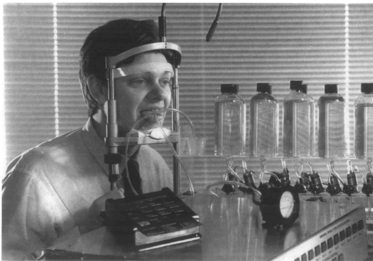
Figure 1 A picture of the University of Pennsylvania Regional Automated Taste Testing System showing the glass stimulation device held to the subject's tongue tip.
